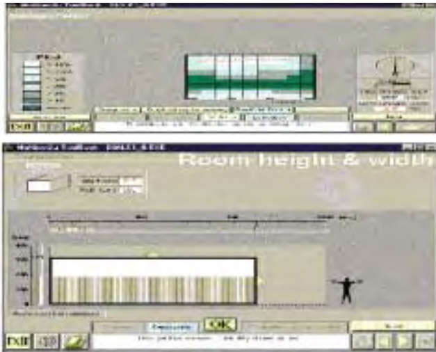
Screen views of the LESO DIAL daylight program showing the menu for room definitions and the calculated daylight factors in the room.
