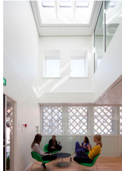
The roof windows have a significant and positive influence on the daylighting level in the building.
