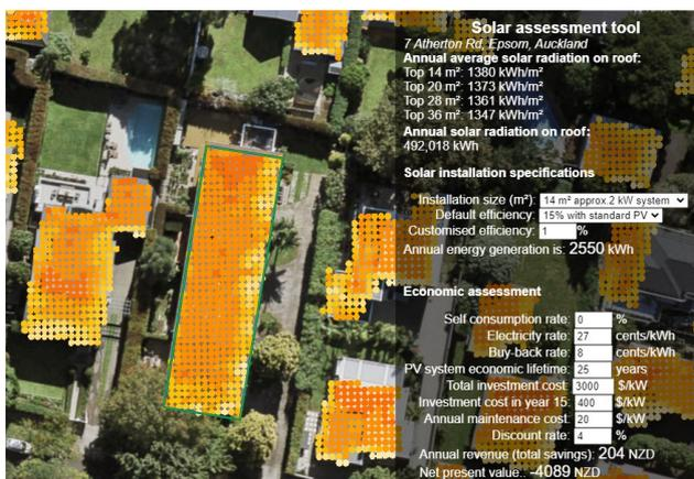
**Figure 6: Auckland Rooftop Solar Energy Potential web platform**
