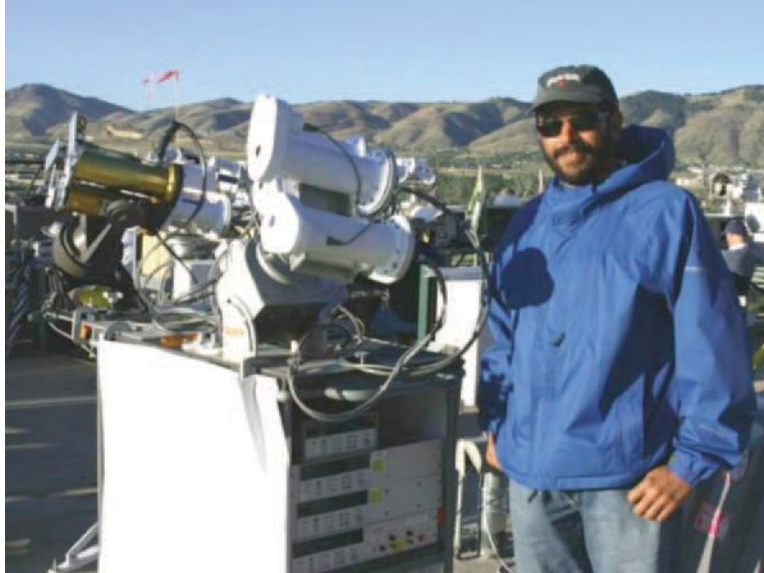
Figure 3-6. Multiple electrically self-calibrating absolute cavity radiometers mounted on solar trackers with control and data acquisition electronics. Photo from NREL
