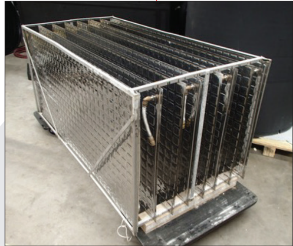
▲ Experimental ice storage heat exchanger using flat plate collectors in stainless steel.
